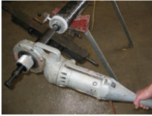
using portable power drive
