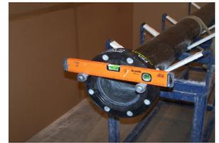
Photo 14 - Check boltholes alignment
