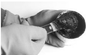
High speed die grinder for sanding sockets. Use drum with 36-60 grit abrasive
