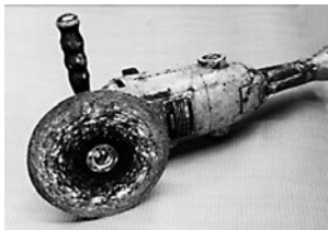
Disk power sander for large diameter pipe. Use 36-60 grit abrasive
