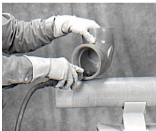
High speed die grinder for sanding sockets. Use drum with 36-60 grit abrasive
