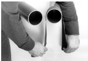
"Shoe Shine" method using Emery cloth of 36-60 grit abrasive
