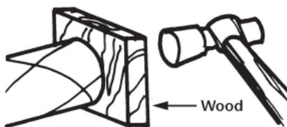
Check lock up by moving a free end of the pipe in an up and down or side to side motion. The movement must be sufficient to move the joint being checked. No movement should be visible in the joint. If any movement exists, the joint is not properly locked up. Avoid excess movement as this could damage the spigot.
