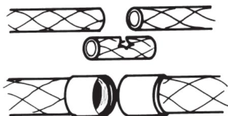
3. If the line cannot be moved sufficiently to install a sleeve coupling or a sleeve coupling spool piece, taper both ends of the pipe and install flanges.
