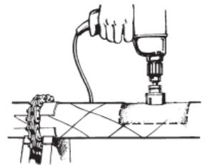
Apply a thick coat of adhesive to the O.D. of the pipe and the I.D. of the saddle, and the edges of the pipe wall exposed by the hole. Place the saddle over the hole and clamp with two hose clamps or a strap clamp. The clamps may be left on after the joint is cured.
