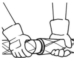
Align and lock the joint. For 2" or smaller pipe, insert the spigot into the bell until surfaces touch, then push and turn at the same time until a lock is achieved. Only a quarter to a half turn is usually needed. On 3"-6" diameter pipe or on fittings, pushing and turning to lock the joint is impractical and driving force must be used. A hammer may be used to assist in joint lock-up. Place a 2x4 board flat across the bell. The first few raps should be light to
