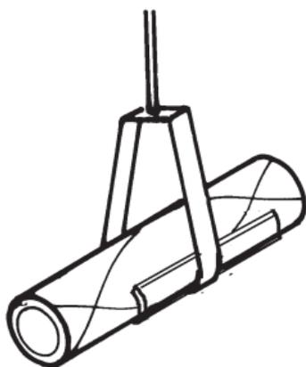
**Pipe Guides** - are rigidly fixed to the supporting structure and allow the pipe to move in the axial direction only. Proper guide placement and spacing are important to ensure proper movement of expansion joints or loops and to prevent buckling of the line.
