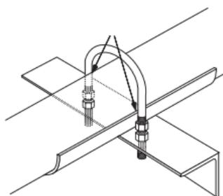
The guiding mechanism should be loose so it will allow free axial movement of the pipe. “U” bolts, double-nutted so they cannot be pulled down tight, are often utilized for guides.
