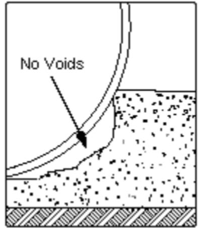
small stones or debris into the pipe wall if they are present in the bedding material. Avoid striking the pipe with tamping equipment as the pipe may be fractured.
