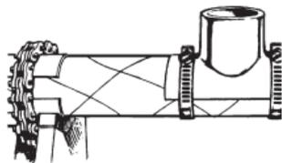
**Installing Reducer Bushings** - Install reducer bushings using a block of wood and a hammer and the same procedures as for bell and spigot pipe. The wood block should be sized to allow the reducer bushing to be counter-sunk in the bell. Some reducer bushings will be counter-sunk before they are actually locked up. For maximum chemical resistance with 8" and larger Green Thread reducer bushings, coat all machined surfaces with adhesive just before assembly.
