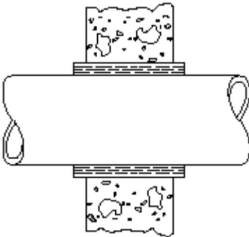
resilient material should be wrapped around the pipe to provide flexibility and prevent contact with the concrete. If bolts are used in the resilient material, care should be taken that the bolts, nuts, or washers cannot come into point load contact with the pipe. Bedding depth under the pipe should be increased to a minimum of 12" or one pipe diameter, whichever is greater, for one pipe joint length away from the concrete.
