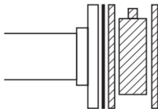
hard spacer ring or steel back-up ring placed between the raised face and the outer edge of the flange to form a full flat face on the mating flange is recommended. The purpose of the spacer is to fill the gap outside the raised face to prevent bolt loads from bending and breaking the fiberglass flange.
