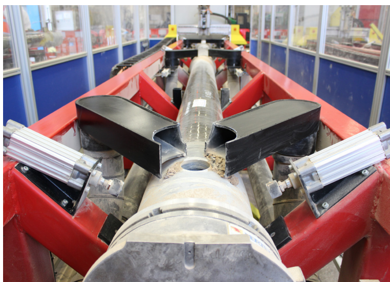
Figure 5. One of two custom CNC machines built to manufacture the pressure vessels to BP's specification parameters while maintaining repeatable quality and production flow.
